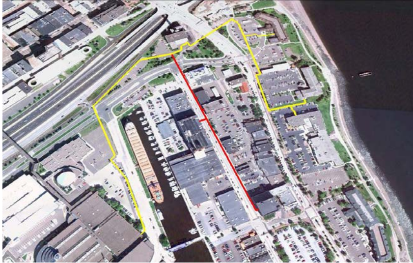
Figure 4.1.2.1: Existing steam (red) and hot water networks (yellow)
