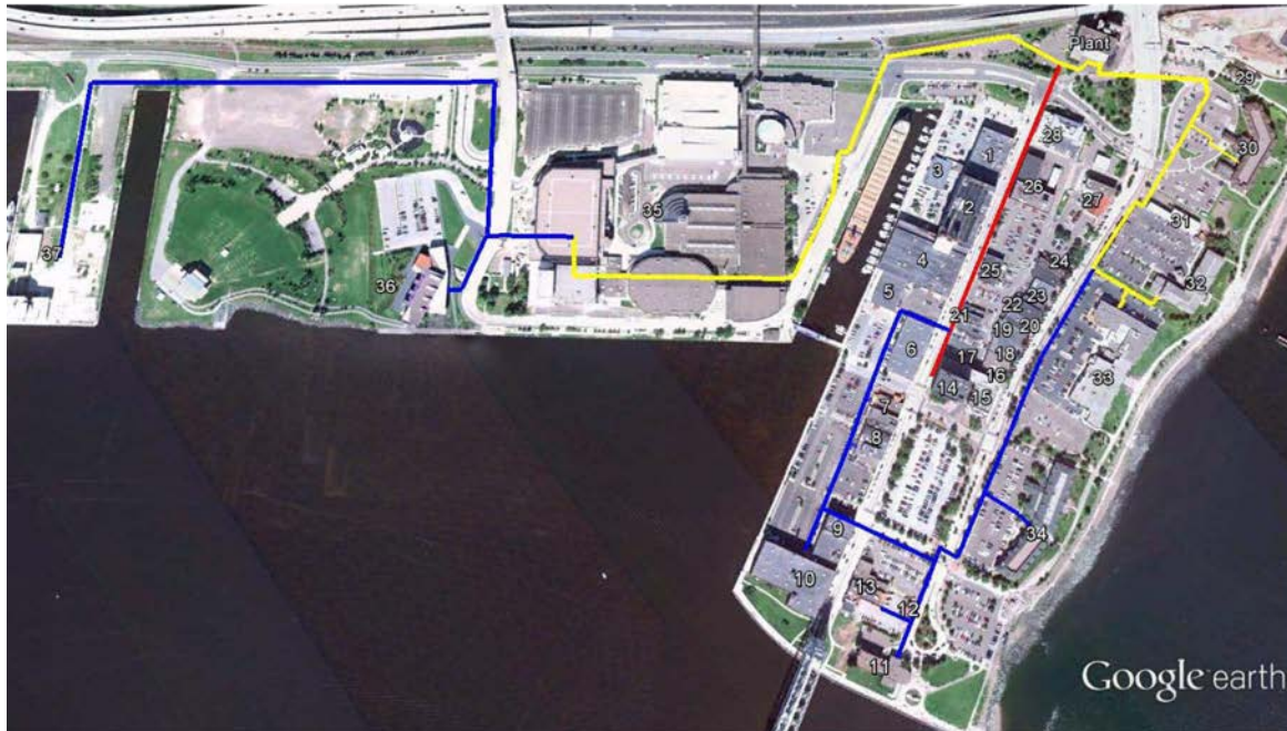
Figure 4.3.1: Full build out hot water distribution network
