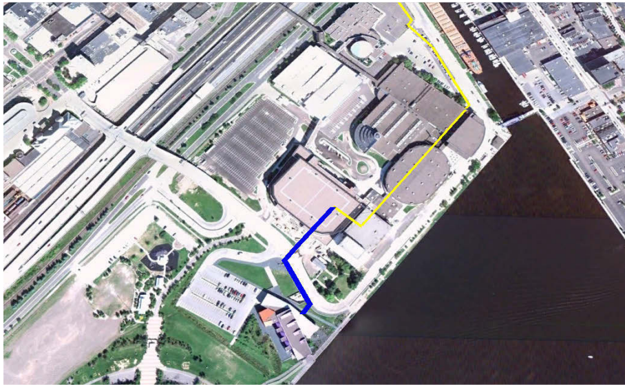
Figure 4.1.2.2: Great Lakes Aquarium hot water extension served through AMSOIL Arena. The pipe routing through DECC and AMSOIL Arena is not actual and has been simplified.
